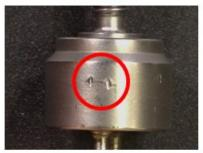
A wide, rough scratch with sharp corners and deformation
