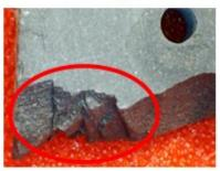
A breaking away of an edge caused by impact from a foreign object
