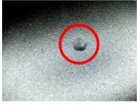
A depression with rounded edges caused by impact with a blunt object
